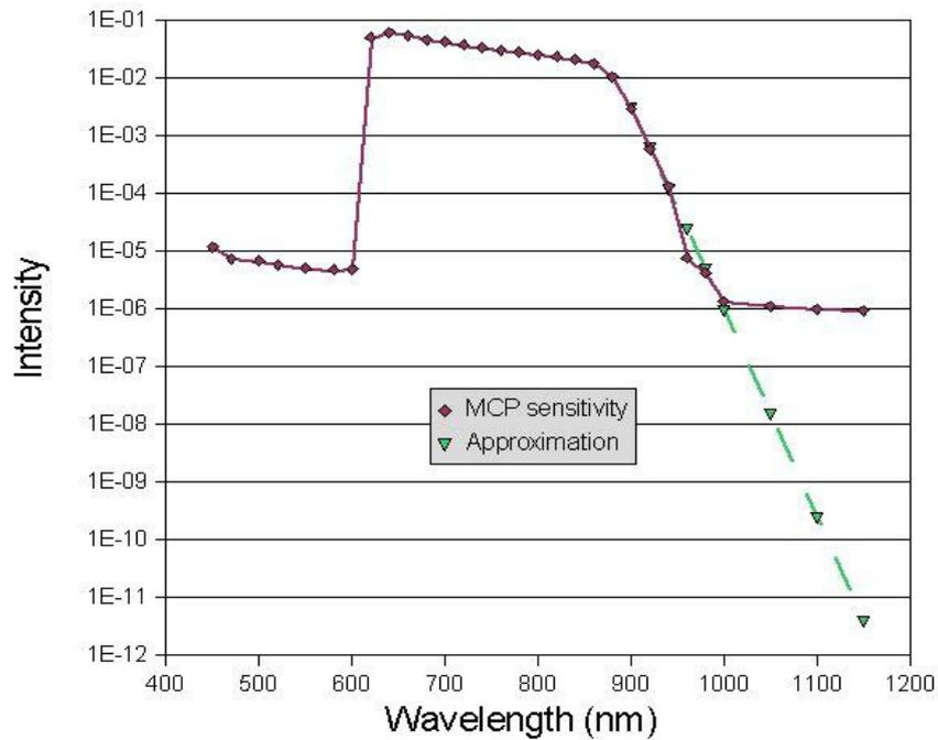
Figure 2. Spectral sensitivity of a typical image intensifier and extrapolation of the curve in the IR range to overcome the light scatter effect inherent to the spectrometer.
