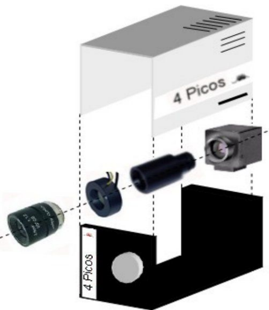
Figure 2. MTF of an ICCD camera ; MTF_{lens} \times MTF_{MCP} \times MTF_{coupling\ lens} \times MTF_{camera} = MTF_{total}
