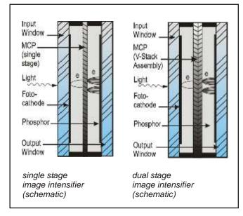
First the incoming photon releases an electron in the photocathode, second the electron is accelerated and amplified to an electron avalanche within the multi-channel plate (MCP), third the accelerated electrons are converted into photons by the phosphor screen.
